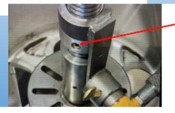
Brass Set Screw – Tightening this set screw with an Allen Wrench locks the Sliding Ring to the Mainshaft. Since the screw is recessed, it will not interfere with the rotation of the Ram Housing, allowing it and the wheel to spin freely while the Ram is held stationary. This allows the Ram to be, used as a reference indicator. In some cases the need for a dial indicator setup can be eliminated.
