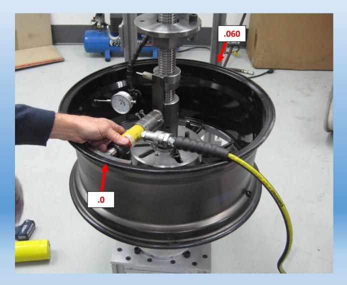
Remember that, when straightening forces are concentrated in the bend location, the wheel is also being torqued downward. This causes the opposite side of the wheel to come up and in slightly, as shown here.
