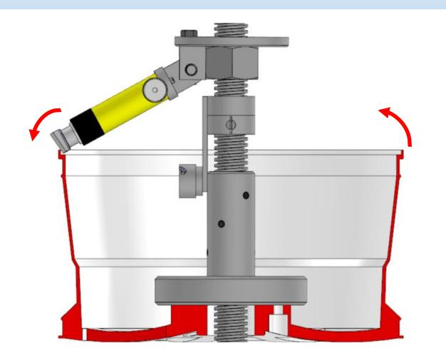
If using 4,000 pounds of pressure to correct a .060" runout at one location has resulted in the .060" moving to a location 180 away, the simplest solution is to set the upper axis at a steep angle and use lighter pressure to press the wheel downward.
