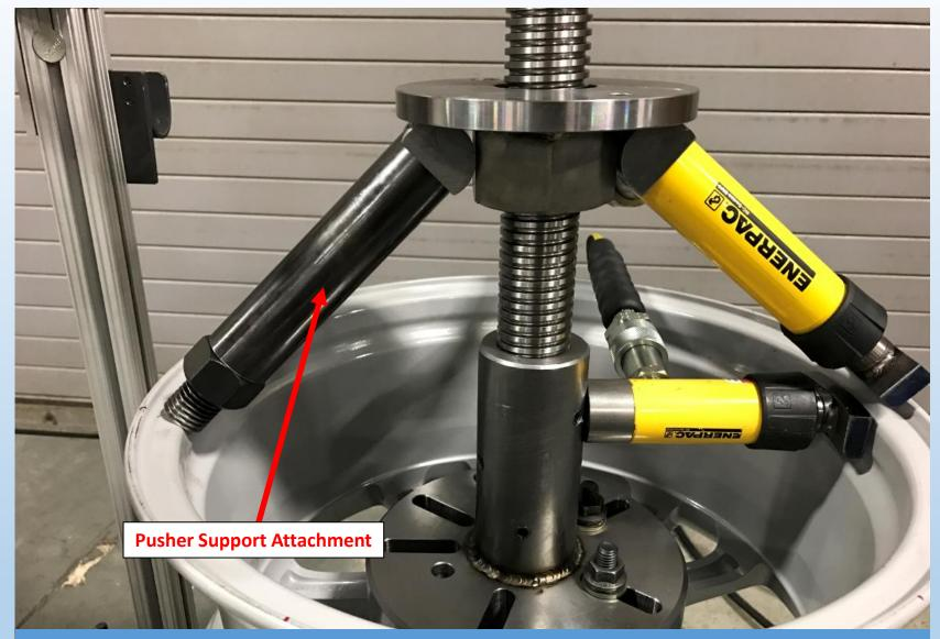
Another strategy to use if lateral torqueing seems to be a problem is to use the Pusher Support Attachment. If it is set up as shown above, it mirrors the position of the upper axis and prevent lateral upward movement of the wheel at the spot 180 degrees from the bend site. The nut only needs to be finger tight at setup, just enough to hold it in position. This attachment will also help support the mainshaft from straightening forces.
