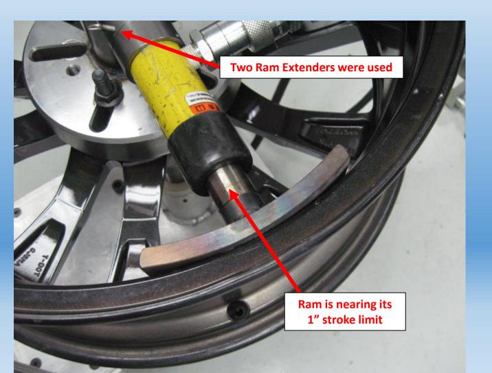
Here a RC51 is being used on a larger rim. Even though two extenders are being used, the Ram has nearly used all of its stroke.
