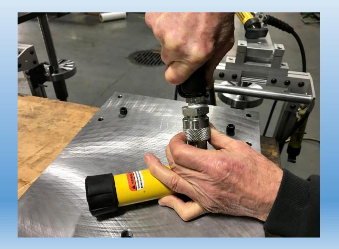
When the male coupler on the end of the Enerpac hose is tightened securely into the female coupler in the Enerpac Ram, the check valve in the Ram is held open so oil can travel both to the Ram from the Pump and back to the Pump from the Ram. The knurled nut needs to be only finger tight to keep the connection secure.
