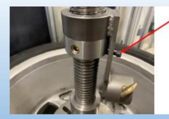
Freefall Bolt - Once you have mounted the attachment on the Mainshaft, you can leave it in place permanently. It will not interfere in straighten setups, even when you don't use it. It is there simply to prevent the Ram Holder from free-falling when the shaft is turned upright. It is not necessary to use this bolt for any other reason so it can be backed off or removed entirely if desired.
