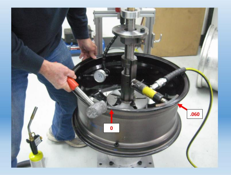
Typical straightening procedures concentrate outward forces at the bend site while using inward impact forces on each side of the bend. Dial indicator measurements will confirm the most positive readings will be at the original bend and the most negative readings will be on each side of the original bend.
