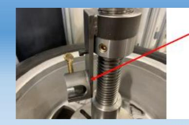
The Ram Housing position shown here is above the Mainshaft Hub. If you are working on an unusually wide wheel and need to position the Hydraulic Ram high on the rim edge, you will need to place a shim, about 3/8" thick behind the flat platen to support it *during pressure applications*. Otherwise, there is a risk of bending it.
