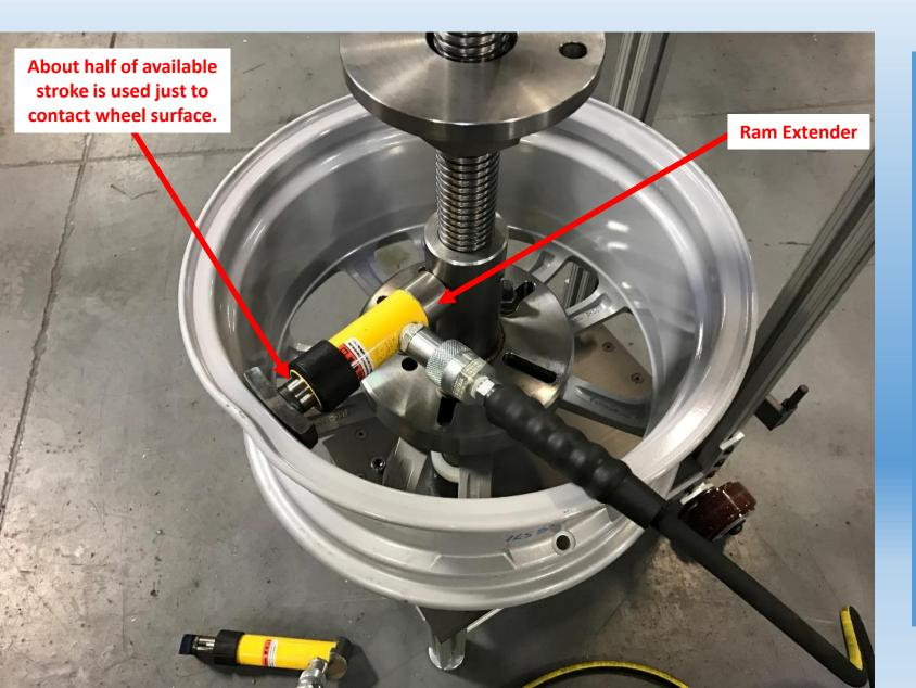
The first of the three most common problems is "False Feedback". The single axis setup shown here is using the standard Enerpac RC51 Ram, which has a 1" stroke. Notice that a Ram Extender has been bolted on the end of the Ram. A magnetic Pusher Spacer could also have been used. Either of those components extend the collapsed length of the Ram by 1".
