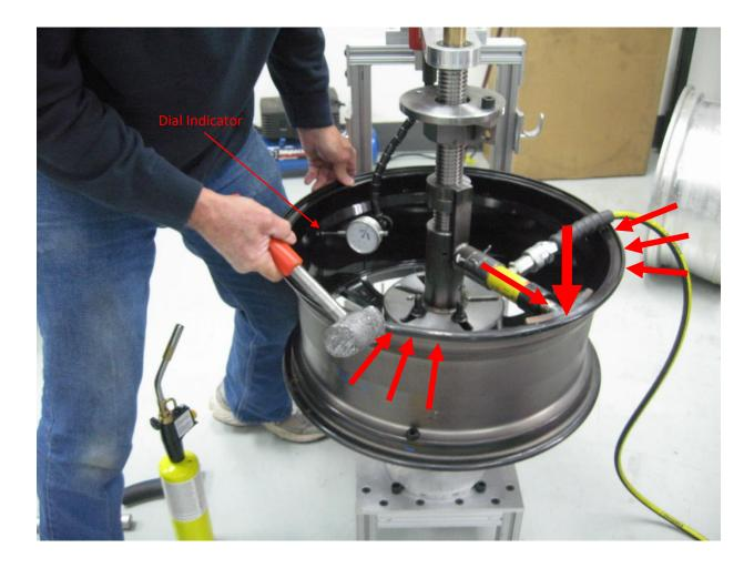
In the After the Dual-Axis hydraulic pressure process has moved the metal back into a shape that looks round to the naked eye, dial indicator readings will reveal the true runout. Once the runout shows the innermost spot on the wheel, the lower axis is placed against that mark and hydraulic pressure is added. Now the final adjustments can begin.
