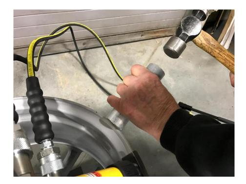
When heavy impact must be applied at a *precise* location, the *Aluminum Drift Punch* is a useful tool. It is a softer grade of aluminum than an alloy wheel so tool marks can be kept at a minimum.
