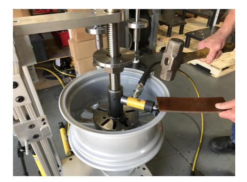
Sometimes the nature and severity of the bend might necessitate the use of *heavier* impact. Here a heavy steel sledge is being used with a piece of urethane to protect the wheel surface. Pieces of soft metal, nylon, wood, leather or even a section of tire side wall can be used to protect the wheel from heavy tool marks.
