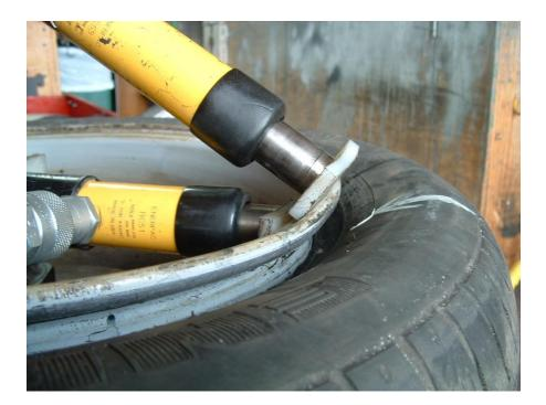
This back-and-forth "massaging" process continued until the physical appearance of the bead was blended nicely with the rest of the wheel. We then began indicator readings.
