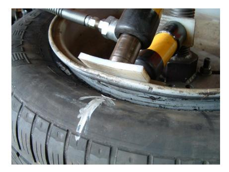
Pressure on the upper ram was next increased to about 3,000 lbs. This dropped the pressure on the inner ram back to about 2,000 lbs. Alternating pressure was added until both rams were reading 3,000 lbs. A progress check was done as the upper ram was slowly removed and the bent area was inspected. When pressure was released from the upper ram, pressure on the inner ram increased to 4,000 lbs. The bend was inspected and appeared OK for additional pressure.
