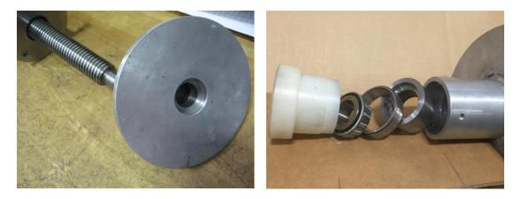
The photo on the left is a view from the underside of the lower Module (325). You can see the edge of the support bushing the Timken bearing cup sits on. The photo on the right shows the entire assembly as it goes together.
