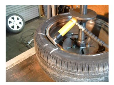
Here a single ram is setup at an angle against the upper part of the wheel weight flange. The rocker (39) is used over the end of the ram as it is secured against the pusher platen (111). Note that a piece of nylon is used at the business end of the ram. When nylon is used in place of a die, the pressure can be focused just as precisely and the surface of the wheel is better protected.
