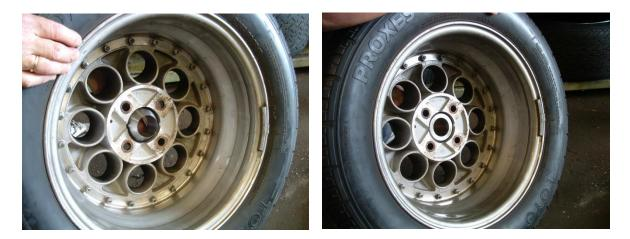
If the centering cone extends too far past the bolting surface of the wheel, it will contact the Mainshaft Platen and interfere with proper centering. The right photo shows that a larger cone will center the wheel properly because it does not protrude through the centerbore.
