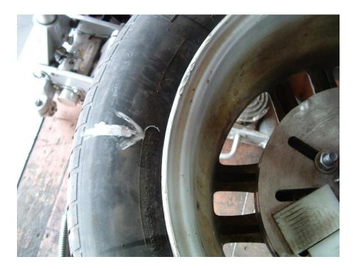
A shot of the wheel, after straightening. The final runout was less than .030" and the total time for the repair was around 20 minutes. It can now be returned to service without the fear of cracking. The fatigue life has been restored to a level equal to an unbent wheel.
