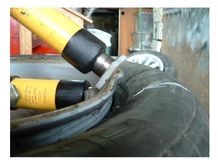
This shot shows how 2 rams were set up on the bend. Instead of using regular dies, both rams were used with small pieces of nylon as pusher dies. After adjusting the ram positions to fit, they were both removed and the area was heated with Mapp Gas and the heat was monitored with a IR Thermometer.
