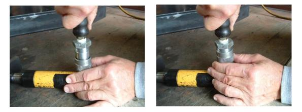
Downward pressure should be continued until the mating surfaces of each coupler meet. At that point, the one-way valve in the ram will be fully open. While holding the coupling fully closed, as shown on the lower right, the knurled nut on the ram can be spun onto the hose quick-connect.
