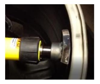
You can lock the lower ram in the desired position without actually contacting the wheel. Then simply swing it out of the way to heat the damaged area. After heating, you can quickly re-position it and commence straightening. The speed of this re-positioning allows you to take advantage of the malleability of the heated metal.
