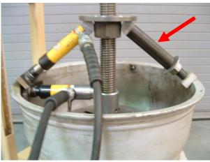
Steep angle setups likely result in more Mainshaft flexing. Also, when a high amount of hydraulic pressure is required more flexing will be evident and a more rigid setup might be required. In such cases, use the Mainshaft Support Attachment, as shown here, is being used on an inboard bend.
