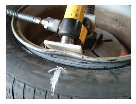
After heating the area for about 2 minutes, the pre-set rams were quickly repositioned in the exact same spots on the wheel. First, the ram in the barrel was loaded to about 2,000 lbs of pressure. The upper ram was then loaded to about 2,000 lbs. This dropped the pressure of the inner ram to well under than 2,000 lbs. The inner ram pressure was then pumped up to 3,000 lbs.
