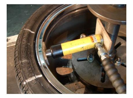
Here a single ram is setup at a low angle inside the barrel of the wheel. The nylon placed against the Mainshaft threads is mainly to protect both the end of the ram and the Mainshaft itself. Nylon is an excellent source for surface protection.
