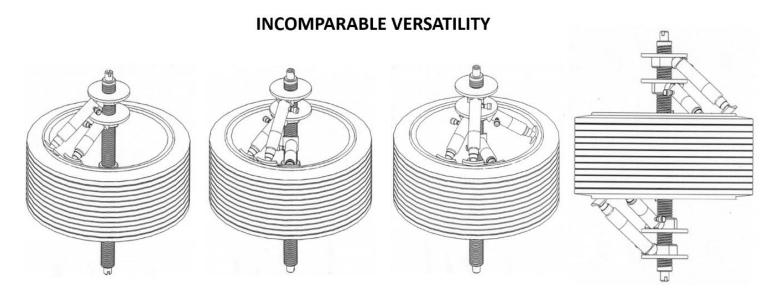
With our patented process, it is possible to create multiple ram setups at varying angles and in separate planes. The setup on the far right shows a unique lateral straightening creation. Needless to say, setups such as these would be very time consuming but these concept drawings depict the incomparable versatility of this machine.
