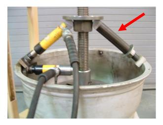
The Mainshaft Support Attachment has the same OD as that of the Enerpac rams, which allows for the attachment of Pusher Spacers and Rockers. It is a simple jackscrew composed of a plain steel tube in which a threaded rod is inserted. The length of the rod and tube can be adjusted by turning the nut. Simply attach a rocker over the end of the support tube and mirror the position of the hydraulic ram on the other side of the Mainshaft.
