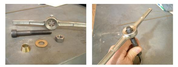
When mounting and dismounting wheels, it is a time saver if the nuts turn freely. If the nuts "hang up" on the bolts it is because the threads have become damaged in some way and they do not ride smoothly inside the nuts. Tossing the bolts among other steel parts or tools can easily damage the threads. Cure this problem using a  $\frac{1}{2}$ "-13 die as a "chaser" over the threads will temporarily restore them to a smooth condition but you should still replace them as soon as possible.
