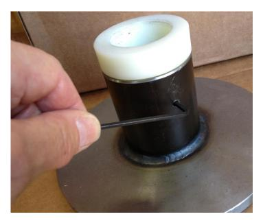
The nylon bushing serves two functions. It protects the mainshaft threads when removing and replacing the lower module. It also keeps the Timken bearing cone in proper position. If the bushing starts to rise up out of the lower module, the bearing cone could become dislodged. If you notice that the bushing is not bottomed out, reposition it properly and retighten the set screws.
