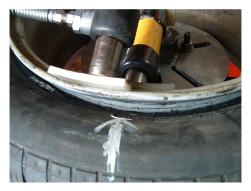
The upper ram was "staggered" to a different plane in the setup and then gradually pumped back up to 3,000 lbs. This dropped the pressure on the inner ram back to about 3,000 lbs. Pressure was alternately and carefully increased while the bent area was observed closely.
