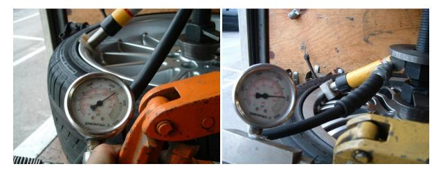
The above two photos show extreme pressure being used on wheels with front bends. When pressure over 5,000psi is used, we recommend the use of the Pusher Support Attachment to support the mainshaft. An excellent view the attachment can be seen on page 11 of this manual.
