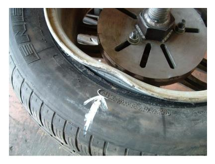
The inboard side of the wheel, showing the bend site. An approximate bend deflection was determined to be over  $\frac{1}{2}$ ". The inboard bead on the tire was then broken to enable maximum heating without having to remove the tire entirely.
