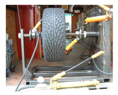
Here two rams are setup on a severe lateral bend that was qualified, using the 180 degree rule. Each ram was set on the high spot on opposite sides of the wheel. Pressure from this setup applies a twist to the center. Lateral runout must be measured and marked before constructing this setup.
