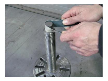
Sanding with aluminum oxide paper or crocus cloth can also be effective. Sometimes the use of lapping compound might even be necessary.
