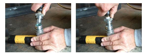
The left photo shows the detent pin on the hose male coupler being positioned over the bore of the ram's female coupler. On the right the detent is being pushed into the bore. As downward pressure is applied, the one-way valve inside the ram will begin opening
