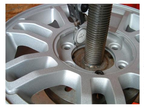
Here is what's called a Test Indicator is set up to check a centerbore. The wheel is slowly spun and tapped into position until the indicator shows the bore is centered.
