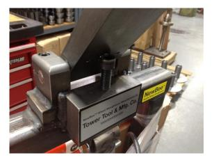
Adjust the torque of the pinch bolts on the Swingarm hinge to regulate the Swingarm motion. The Swingarm should remain in position when parked at a 45 degree angle. If the Swingarm is opened for a long period of time, it is always a good idea to install the Safety Bolt.
