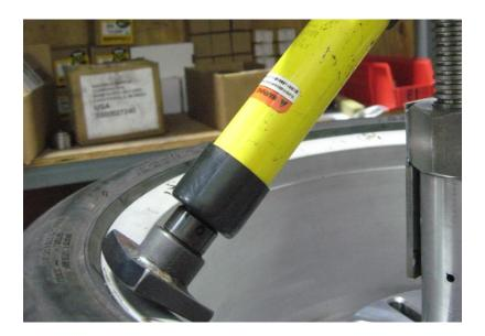
A steep angle single axis setup enables the operator to exert both downward and outward pressure to correct lateral movement. Very little pressure is needed to correct slight lateral runout. To see how the machine can be used to correct a severe lateral bend, refer to page 21 of this manual.
