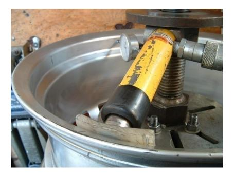
Sometimes, because of the design of the wheel, it is necessary to keep a slight angle on the ram to prevent it from popping out when using nylon. Here a low setup is shown on a wheel that is built with a more profound outward angle under the inboard flange.
