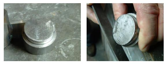
If the edges of the stacking surfaces become damaged, simply remove the damage with a fine flat file until the spacers stack smoothly and fit properly on the Enerpac rams.
