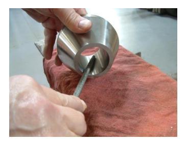
If the inside edges of the cones become damaged, the easiest way to repair them is to use a rat-tail or half-round file. Simply take very light passes with the file to flatten out the dents. Use a fine grade of file. Never use a coarse file to do these types of repairs.
