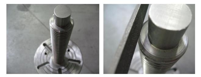
The photo on the left shows the lead thread on the end of the mainshaft, which can become very thin. If this thread becomes damaged it can cause the nut to snag on your shaft. The easiest way to take care of this problem simply to reduce the size of the lead thread by filing down the thinnest part so that it cannot get caught inside the nut.
