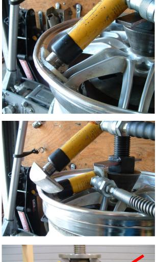
A steep angle is shown over the spokes on an outboard setup. Either a die or a piece of nylon (as shown) can be used against the bent surface. Type and severity of the bend and operator experience will influence setup choices.
