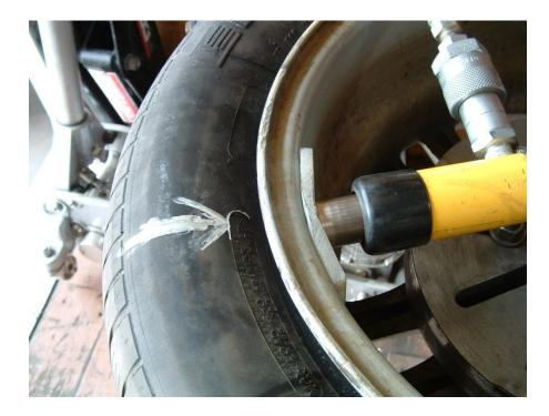
After the bead looked symmetrical, both rams were removed and the dial indicator was mounted. After a runout measurement was taken, a single ram was then setup in the barrel of the wheel with a piece of nylon to complete the final touches. This setup was chosen so as to apply the most focused pressure on the bend to achieve the final roundness desired.
