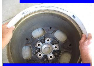
First, place the template tightly against the unbent side of the wheel, as shown here.
