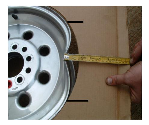
In the above example a piece of cardboard was cut to the true arc of the wheel and then placed against the bend area. The width and depth of the bend can then be easily measured. Without such a true comparison device, the measurements can result in false values and inaccurate acceptance criteria assessments. The most misleading measurement will frequently result while attempting to measure the width of a bend.
