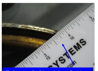
Next measure the distance between these two marks straight across the wheel. The distance shown here measures out at 15 3/4".
