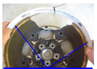
Now turn the wheel around to the bent side and make two marks straight across the bend site 15 3/4" apart, as shown here.
