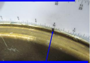
Next place a mark on each side of the wheel at the 10-inch measurement on the template.
