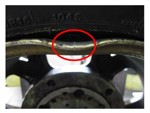
Once the damaged area is clean, some cracks are easily visible to the naked eye. In such a case, dye penetrant inspection is obviously not necessary.
