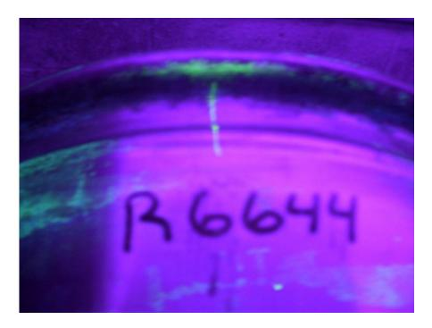
The crack was not visible until inspected under a black or ultra-violet light, using a special fluorescent dye penetrant. The dye is applied to the area and, after the dye has had time to penetrate the surface of the metal. Shined from about 4 inches away, the UV light will detect any dye remaining in even the slightest of surface cracks. Avoid trying this process in direct sunlight. The darker the conditions the better it will work.
