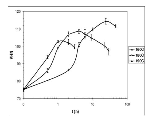
A356-T6 material is solution heat treated at 1000 degrees F for 6 hours then quenched and subsequently artificially aged at three different reference temperatures. The goal is to get near the maximum Vickers Hardness (VHN) without going over the top. The following explain the sensitivity of the hardening process relative to time at temperature.
